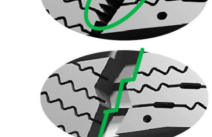
Stepped Snow Shovel Design in Z-Type Pattern Grooves makes sure tire and road are stay attached, enhanced grip ability.
